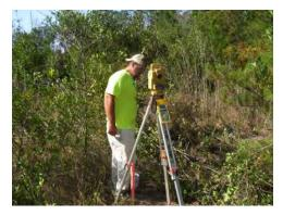
A detailed survey of the construction site should be performed by a qualified surveyor prior to grading-plan development. This survey should include existing topographic information at the site including existing elevations, existing drainage patterns, locations of existing overhead and underground utilities, and construction-limit boundaries.
