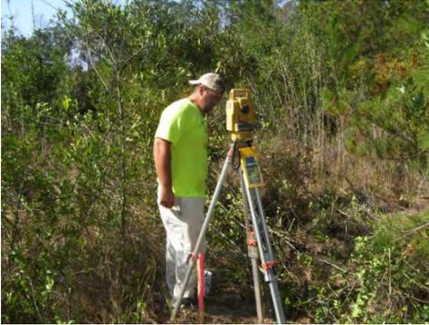
A detailed survey of the construction site should be performed by a qualified surveyor prior to grading-plan development. This survey should include existing topographic information at the site including existing elevations, existing drainage patterns, locations of existing overhead and underground utilities, and construction-limit boundaries.
