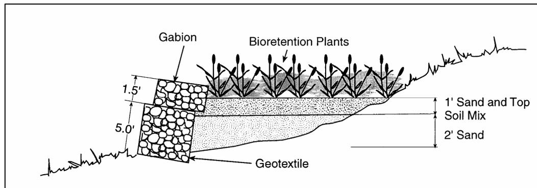
Figure 8 Bioretention Terrace Suitable for Use on Slopes 10-20%
