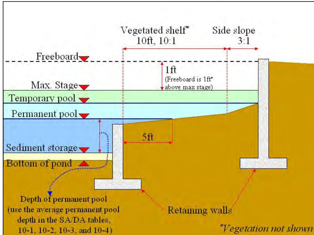
Figure 1 Alternative Wet Pond Design: Retaining Wall Option
