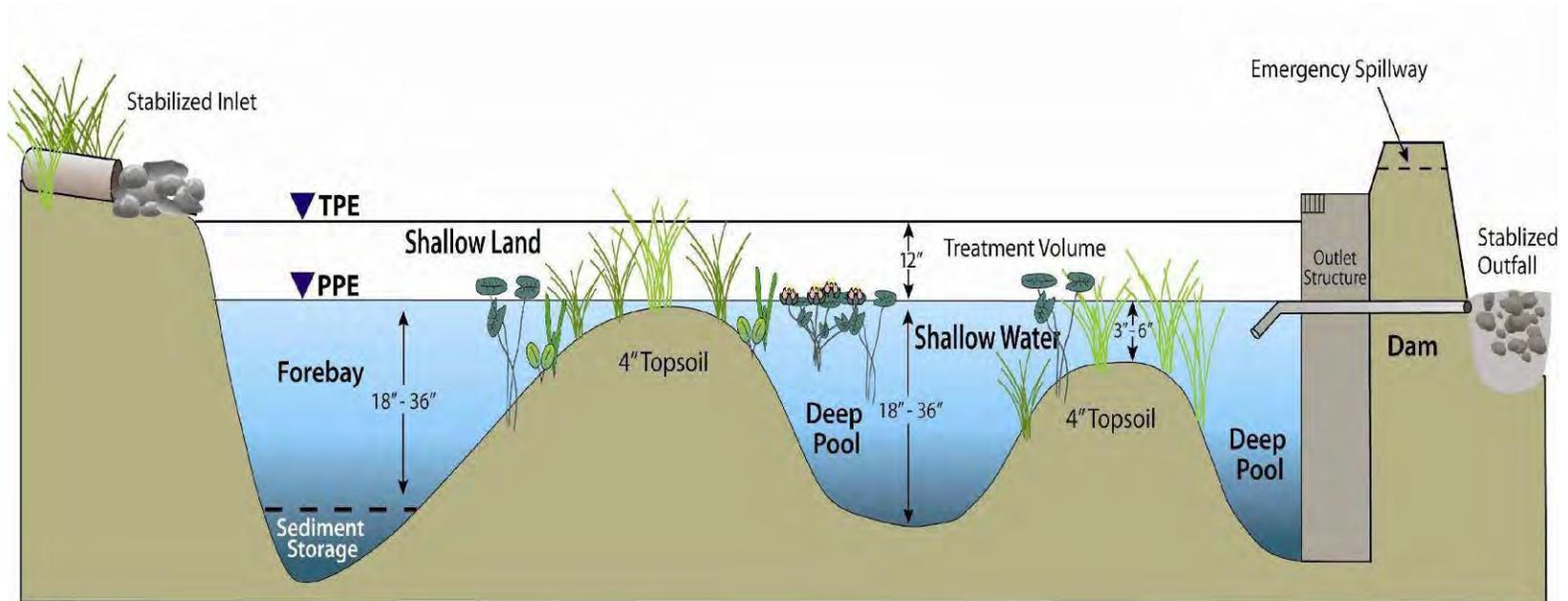
Note: Depending on site soils and groundwater elevations, a clay or synthetic liner may be required to maintain PPE at design elevation.
