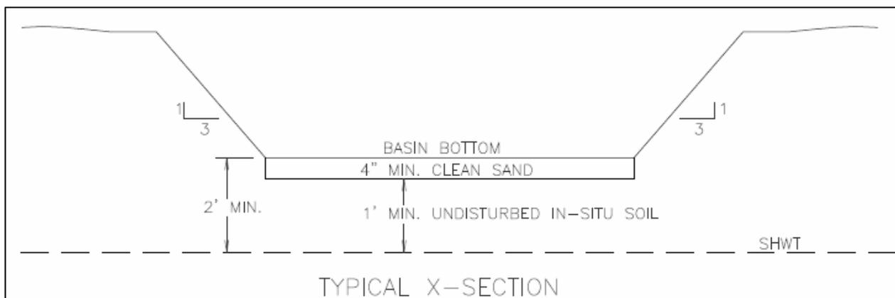
Figure 1 Typical Infiltration Basin: Cross Section
