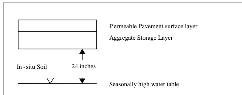
Figure 1 Schematic of Water Table Design Constraint
