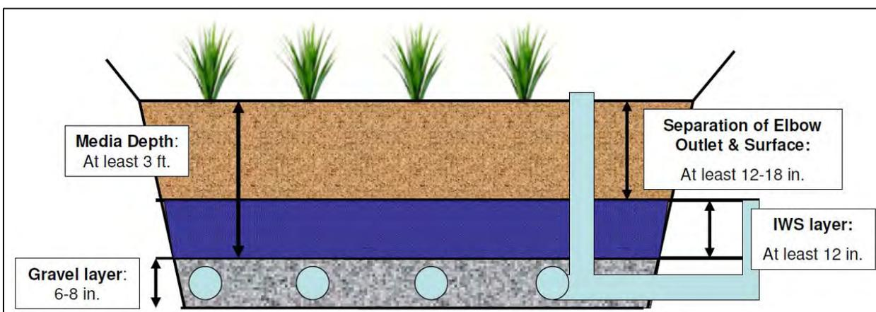
Figure 6 Bioretention Cell showing IWS Zones (Source: NCDENR)
