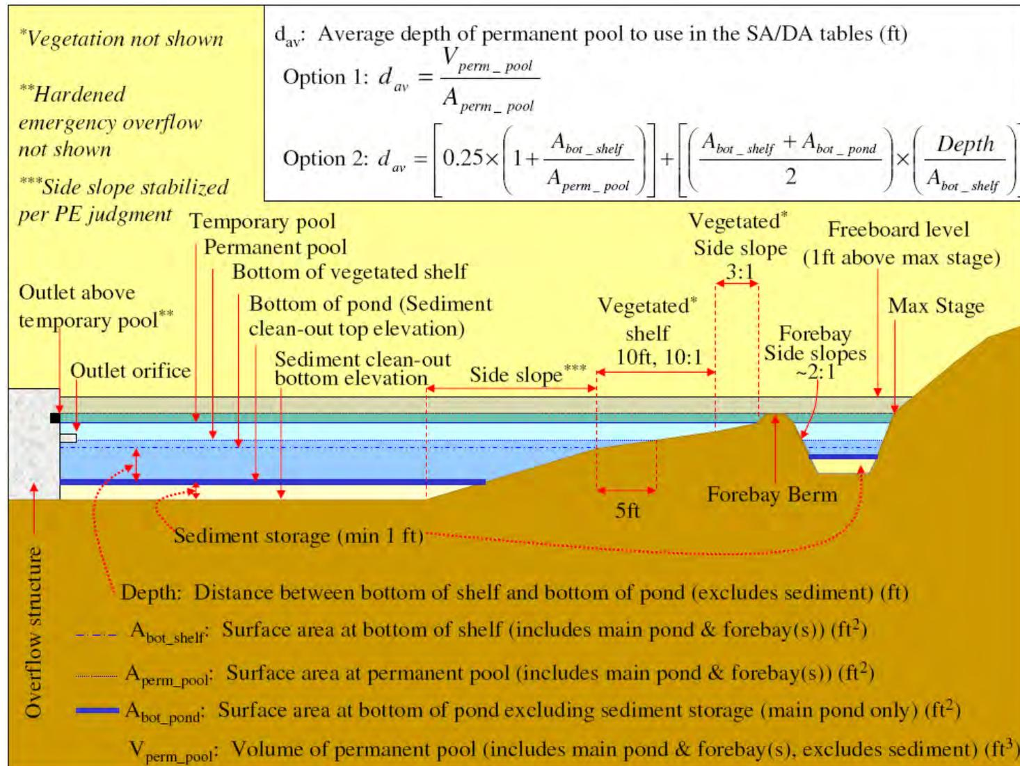
Figure 2 Basic Wet Detention Basin Elements: Cross Section
