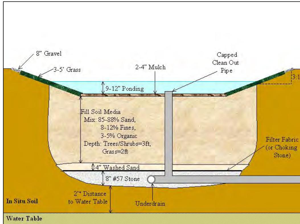
Figure 9: Bioretention Conceptual Layout: Cross-Section (Source: NCDENR)
