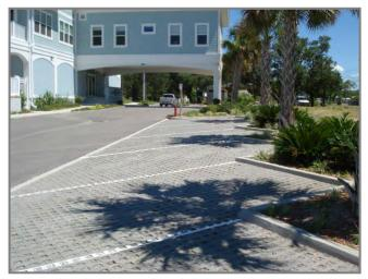
stalls to treat runoff from adjacent impermeable pavements and roofs. This design economizes PICP installation costs while providing sufficient treatment area for the runoff generated from impervious surfaces. Inlets can be places in the PICP to accommodate overflows from extreme storms. The stormwater volume to be captured, stored, infiltrated, or harvested determines the PICP scale required.
