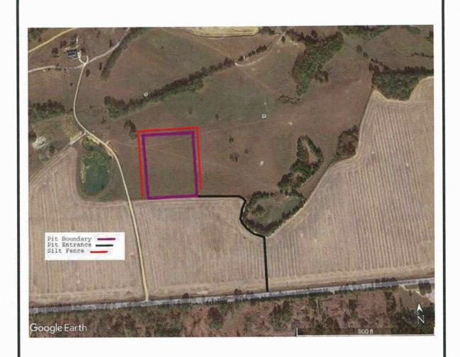
Topsoil to be stripped and stockpiled along perimeter of pit area. Upstream storm water runoff to be diverted around pit area through use of berms. Storm water runoff within pit area to be collected in silt fence prior to exiting mine footprint.
