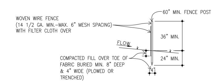
WIRE BACKING NOT REQUIRED ON SILT FENCE
