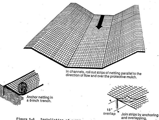
Figure 5-6 Installation of netting and matting.
