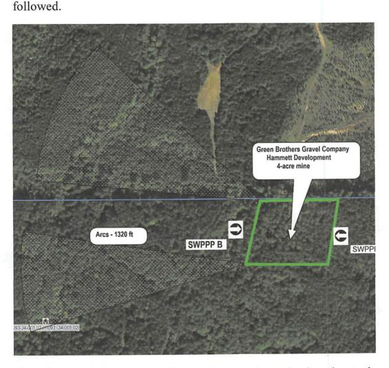
The mine area is located on a ridge, with areas lower in elevation to the east and west. We will monitor SWPPP A and B for any silt or mining material buildup. In addition, we will monitor the area south of the mine, as well as along the access road to ensure no mining or runoff material transgresses the property line.
