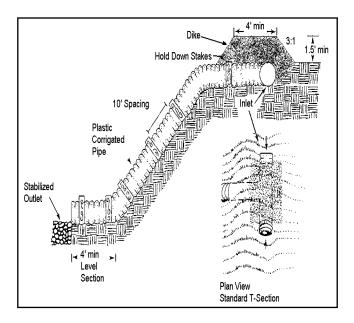
O Slope breaks, diversions or benches, are used to reduce the slope length of a cut or fill to minimize rill erosion and prevent gullying. Drainage area should be less than one (1) acre.
