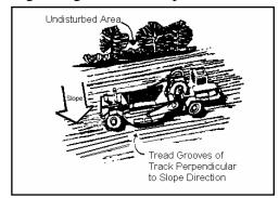
Out slopes that will not be mowed can either be "stair-stepped" or grooved. If stair-step grading, the horizontal portion of each step must be longer than the vertical portion and should be sloped into the vertical portion. Individual vertical cuts should be no higher than 24 inches or 36 inches if the material is rocky.
