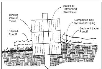
o Gaps between bales shall be wedged with straw. Loose straw scattered immediately uphill increases barrier efficiency. Under no circumstances should straw bale barriers be constructed in live streams. For minor dry swales, the end bale bottoms shall be higher than the middle bale top to assure runoff will not flow around the barrier. Repair
