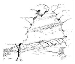
Riprap outlet protection is placed at the outlet end of culverts or channels to reduce the depth, velocity and energy of water so that the flow will not erode the receiving downstream reach.
