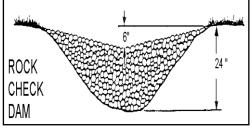
accumulate and should be removed from behind the check dams when it reaches one half the dam height. Erosion around dam edges should be corrected immediately, ensuring that the dam center is six (6) inches lower than the edges. In grass-lined
