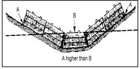
damaged bales, end runs and undercutting. Remove sediment when it reaches one-half (1/2) barrier height. When upslope areas are stabilized, remove bales and grade, seed and mulch barrier line.
