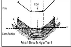
Straw bale barriers are also used on small disturbed areas to capture sediment from sheet flow. The drainage area must be restricted to 1/8 acre per 100 feet of barrier. Maximum gradient behind the barrier is three horizontal to one vertical (3:1). The barrier must be located so that
