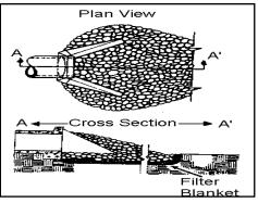
Check dams are small dams constructed across swales or drainage ditches to reduce flow velocity and erosion. The purpose of a check dam is to prevent erosion of the swale or drainage ditch. They are not
