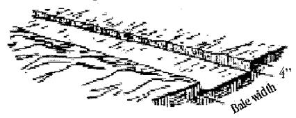
2) Place and stake the bales with 2 steel pickets or 2"x2" stakes. The first stake should be angled toward the previously laid bale. Trim or cap tops of stakes.
